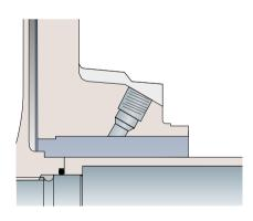
Standard Bore Box accommodates most single component and cartridge mechanical seals as well as standard packing.
