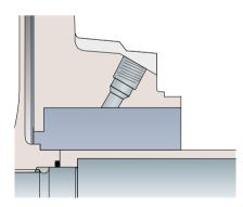
Large Bore Box is designed for seals with large gland bolt circles. It accommodates most single and double mechanical seals, as well as cartridge or component seals. The oversized chamber helps reduce running temperatures while improving lubrication and circulation.
