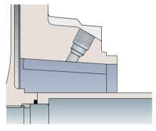
Tapered and Ribbed Bore Box features a seal chamber designed for single and double mechanical seals. The cast ribs inside the stuffing box convert circular flow into axial flow, reducing wear and extending longevity.
